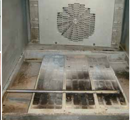
The baking chamber after the covering plates were removed and the nozzle fittings are exposed. Only heat residue and a very light and thin limescale layer are visible on the sides and on the edging at the back.
