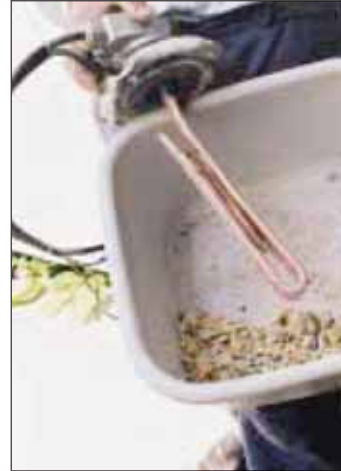
A Before testing, heating rod after 12 months of use: the limescale was hard as stone
