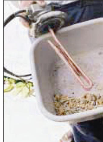
A Before testing, heating rod after 12 months of use: the limescale was hard as stone
